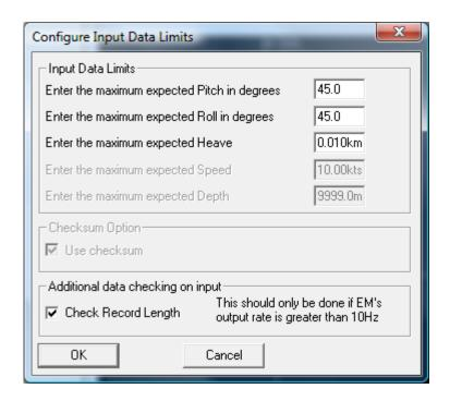
You can enter the maximum expected value for pitch, roll and heave. If the absolute value of the decoded pitch, roll or heave, in a given message is greater than the respective entered maximum expected value, the data is flagged and none of the data in that message is passed to the vehicle. The status is shown in the I/O Device window with an asterisk next to the specific data that failed the test. If heading is included in the message, it is also verified to be >= 0 and < 360.
