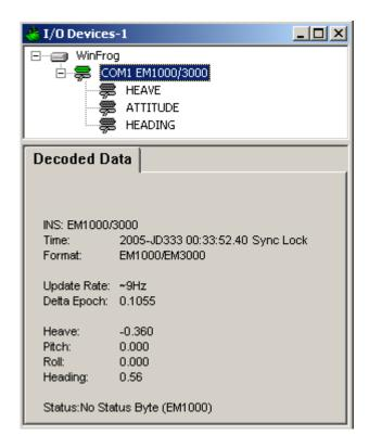
WinFrog will accept two different telegram formats for this device, the EM1000 and the EM3000. The format is automatically detected and decoded.
